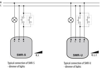
Warning: it cannot be used for fluorescent lights and energy saving lights! SMR-U: It is not allowed to connect together loads of inductive and capacitive type at the same time
